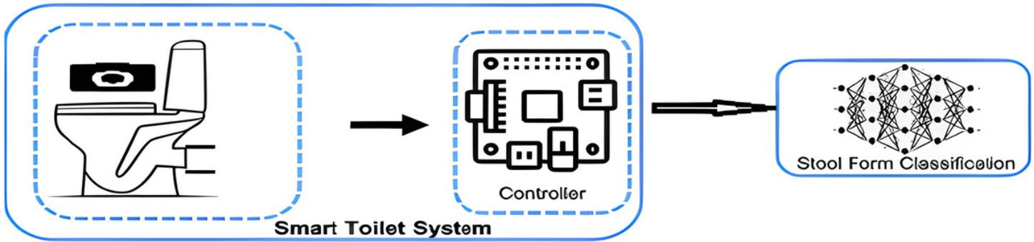
Figure 3: Framework for stool image analysis in a smart toilet system. (a) Images are captured when the stool is in the toilet pot (b) Images are processed by the controller and fed to machine learning algorithms.
