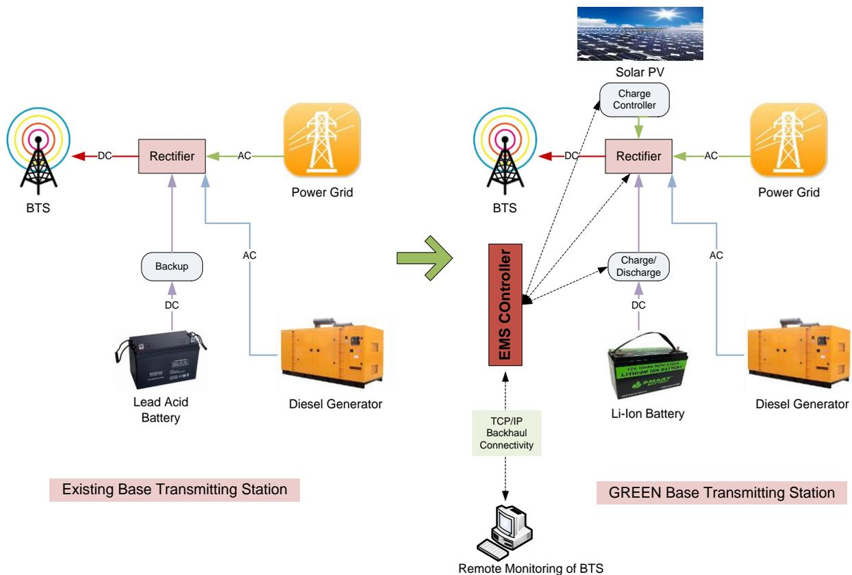
This combination of various inputs and using the same effectively can help reduce the dependency on diesel and CO2 emission.
