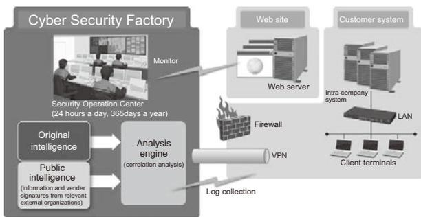
Fig. 5 Security monitoring architecture.
