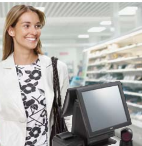
Standard Model 15" operator display, 12" customer display, thermal printer, stand barcode scanner
