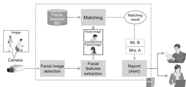
Fig. 2 System image of face recognition.
