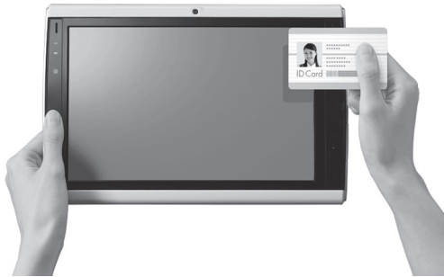
Photo 1 Size reduction of the NFC module enabling IC card authentication on a tablet front panel.
